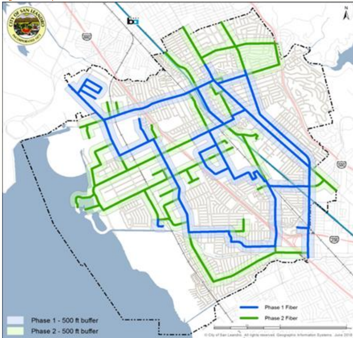
Figure 73. Proposed Fiber Network – Phase 1 and 2: Full Size
